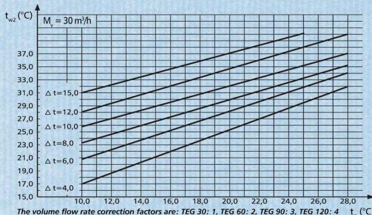
When making use of the diagrams the volume flow rate correction factors of different operational conditions, please, consult our company.
